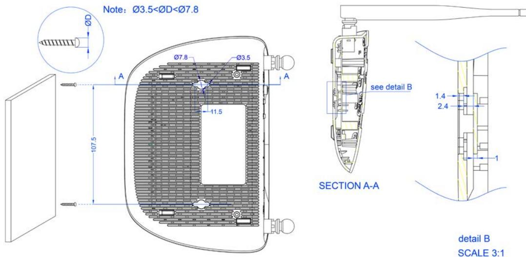
Figure 2-1 Wall-mount install
